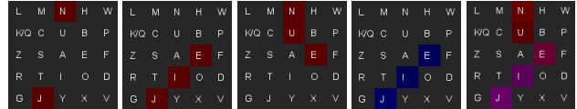
Figure 1. Constructing a string-map image. The first four images show the sub-maps that are summed to construct the final string-map image (right-most image) for the example word “JEN”.
